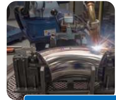
Robotic CMT welding
