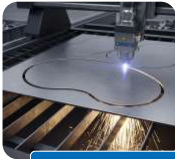
Laser cutting of blanks
