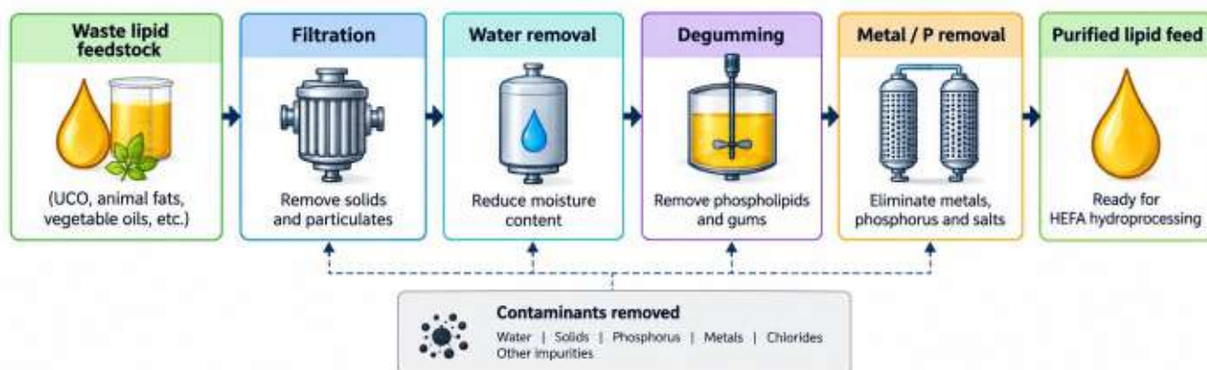
Figure 1. Feedstock pretreatment pathway for waste oils prior to HEFA hydroprocessing.
