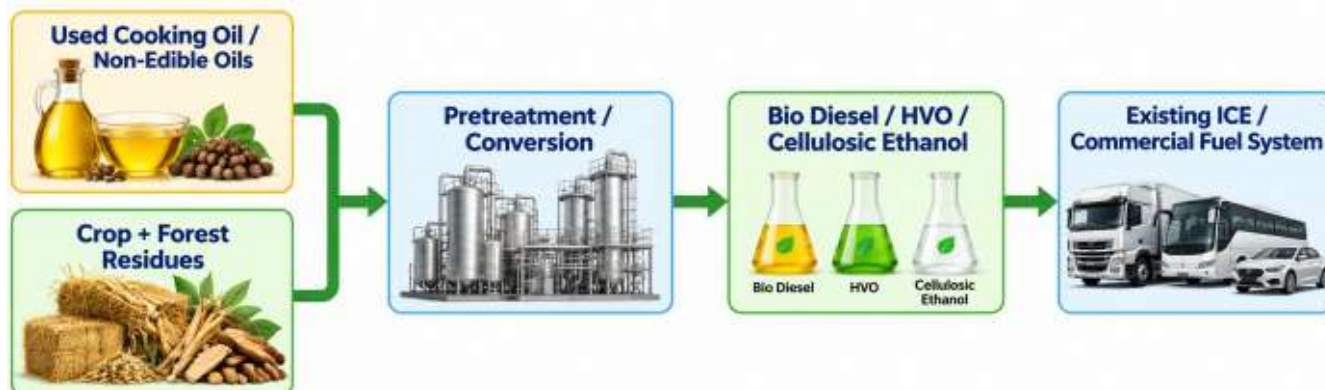
Figure 8. Advancing biofuels can widen the feedstock base and use existing vehicle/fuel assets. Conceptual diagram informed by IEA advanced-biofuel research.
