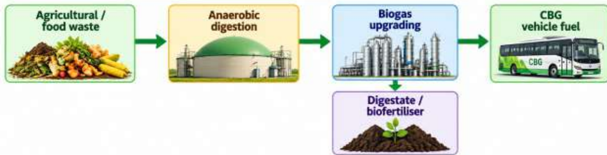
Figure 6. CBG can turn organic residues into vehicle fuel and biofertiliser. Conceptual diagram; Indian CBG blending obligations sourced from PNGRB.
