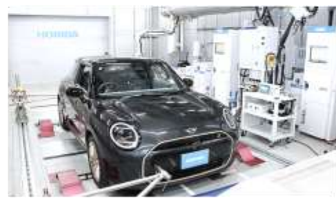
Automated BEV Range Test
