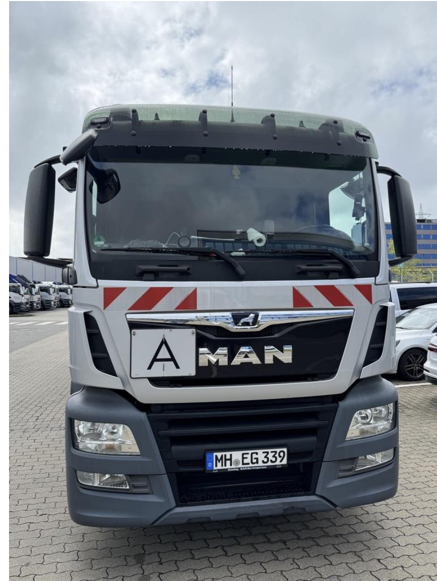
Garbage Truck Owner: MEG V_H = 10,5 \text{ l} P = 235 \text{ kW} Diesel, EURO VI c
