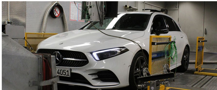
The Mercedes A200 on the ADAC exhaust test bench
