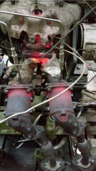
Catalytic Converter size : Dia 40 \* 60 or 74.5 mm L
