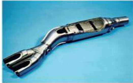
Underfloor catalyst with electrically heated Catalyst EHC
