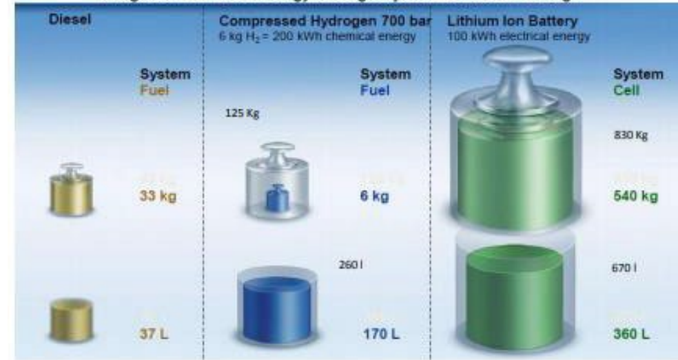
Weight & Volume of Energy Storage System for 500 km Range
