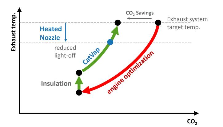
**Efficient Exhaust Heating will improve CO<sub>2</sub> Emission.**
