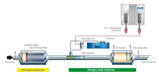
DOC: for active and passive regeneration →increase of temperature by fuel dosing or/and measures
