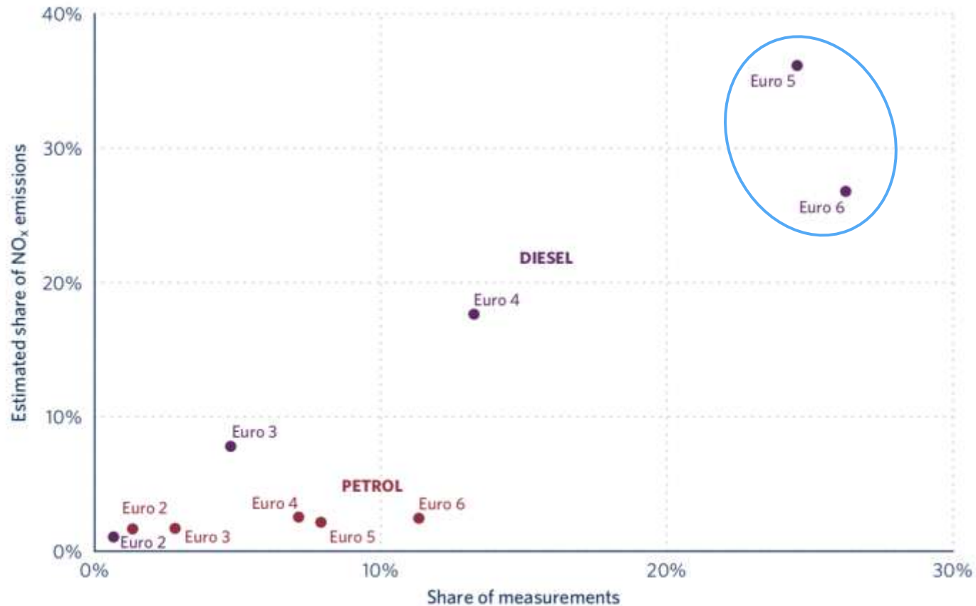
Figure 11. Estimated share of annual NO x emissions from passenger cars and respective share of remote sensing measurements in Paris, differentiated by Euro standard and fuel type.
