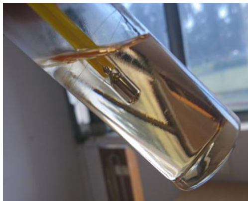
M15 blend+3%CS at -10°C Moisture-- 1200 PPM) - No Phase separation
