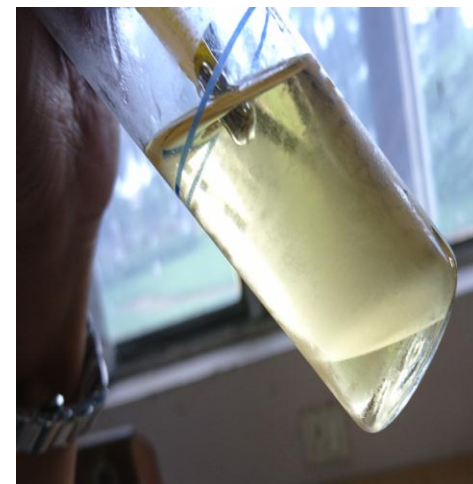
M15 at -10°C ( Moisture-- 600 PPM) --Phase separation
