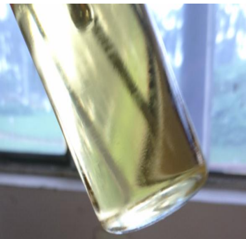
Gasoline as such at -10°C (moisture -80 ppm) -No Phase separation
