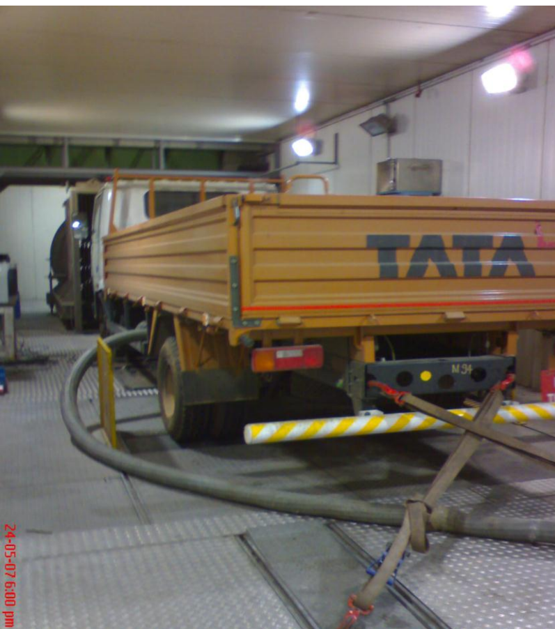
Climatic chamber testing at Indian Oil R&D
