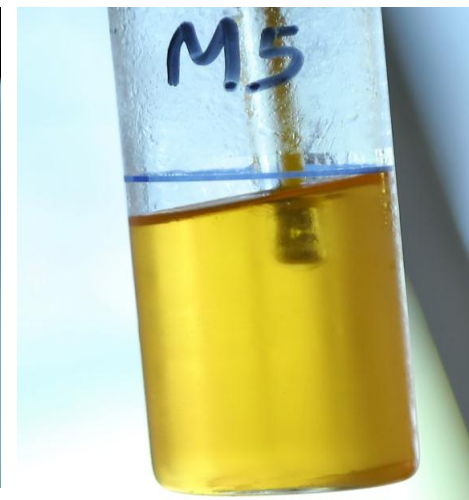
M 5 at -10°C ( moisture-150ppm ---Phase separation
