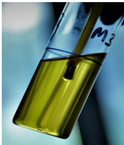
M3 at -10°C ( moisture-150ppm Phase separation
