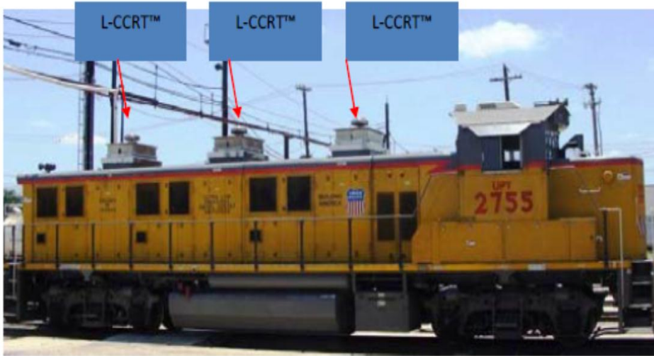
Passive DPF Retrofits on Tier 2 Gen-Set Switcher Loco
