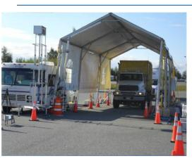
Trucks drive through an engineered portable tent and emissions are measured.
