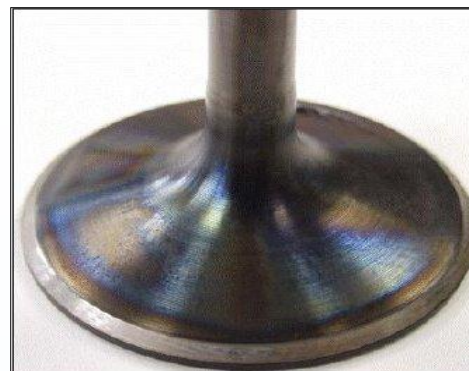
Clean Inlet Valve with additive treated Fuel
