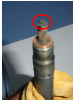
Heavily Scored Injector Pintle with Untreated Fuel
