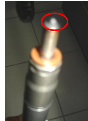
Clean Injector Pintle with additive treated Fuel
