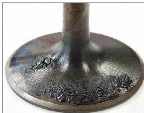
Heavily Scored Inlet Valve with Untreated Fuel
