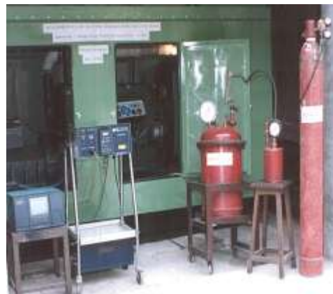
SIX CYLINDER HYDROGEN – DIESEL DUAL ENGINE GENSET – (Ashok Leyland Engine)
