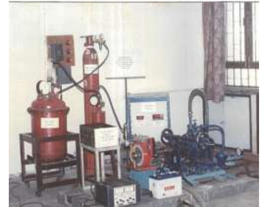
Neat Hydrogen-fuelled S.I. Engine Genset
