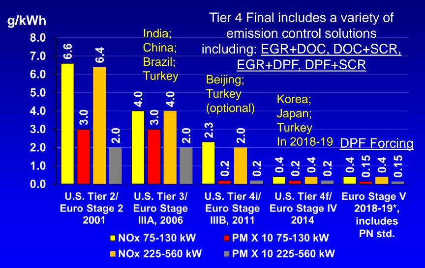
Notes: Change from steady-state cycle to NRTC starting with U.S. Tier 4i/Euro Stage IIIB (5% cold transient weighting in U.S.; 10% in EU & Japan)
