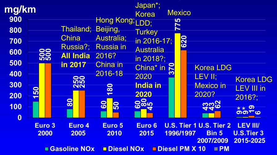
Euro 5+ (2011) and 6 include 6 X 10<sup>11</sup>/km particle number limit for diesels; Euro 6c starting late 2017 includes same PN limit for gasoline direct injection engines, WLTC, & start of RDE;
