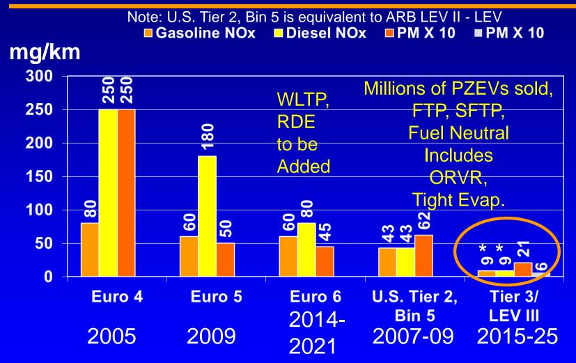
Euro 5+ (2011) and 6 include 6 X 10<sup>11</sup>/km PN limit for diesels; Euro 6c includes same PN limit for GDI (with 3 year delay); Euro 6 PM mass limit uses revised PMP mass protocol; \* LEV III has a 30 mg/mi (19 mg/km) NMOG+NOx fleet ave. in 2025
