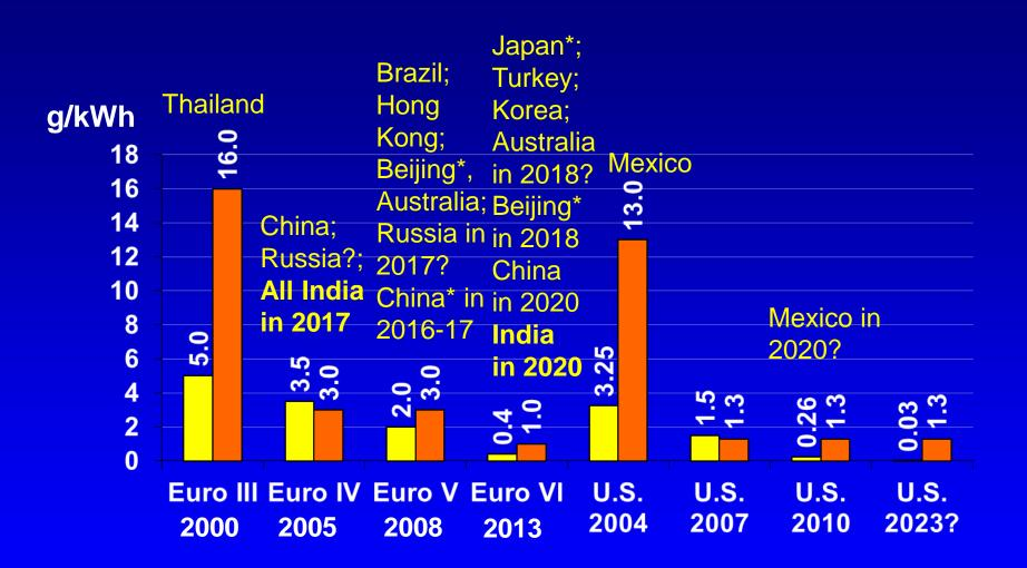
□ Diesel NOx □ Diesel PM X 100
