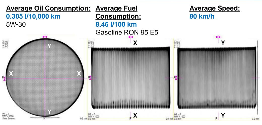
No cracks was observed in GPF. Deposits of ash were detected mainly at the rear of GPF. Ash amount determined after 160,000 km -> 22 g ash.
