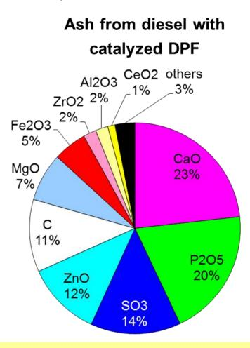
Gasoline engine oil ash components are similar to diesel reference oil ash. Ca and P are major components from oil.
