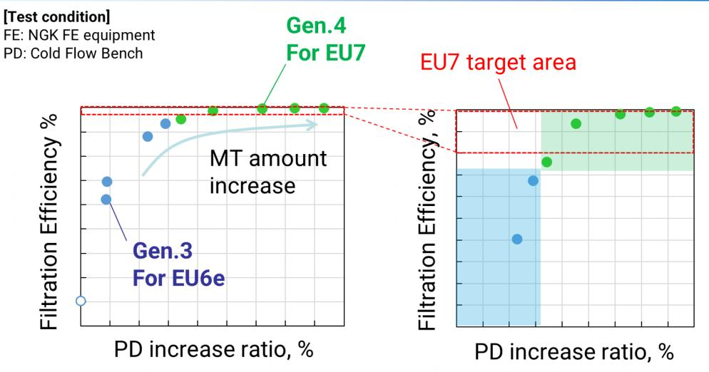
Applying optimized MT condition, MT GPF can achieve EU7 FE target.
