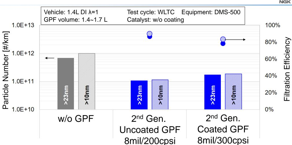
PN emissions will increase by extending measurement range of PN size from >23 to >10nm. GPFs show higher filtration efficiency when counting >10nm particle size.
