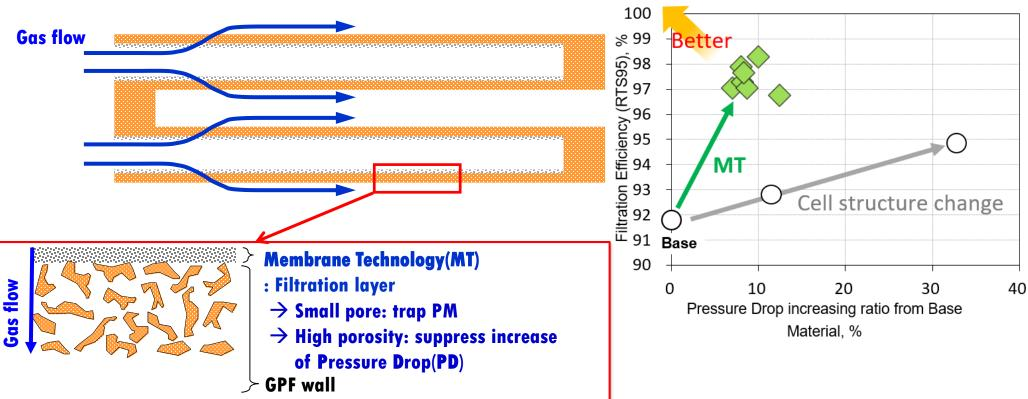
GPF base design change for high FE requirement causes pressure drop increase drastically. MT improves FE with minimum pressure drop increase.
