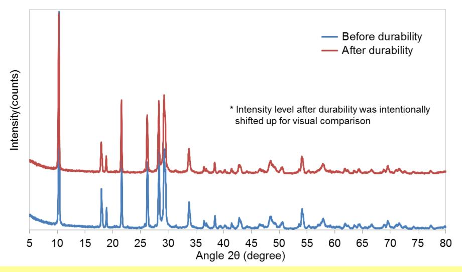
No change for Cordierite crystalline structure after 160,000 km. -> No reaction with ash occurred during this durability test.
