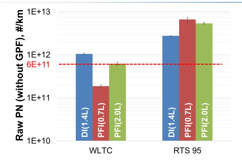
In some driving condition, PFI vehicle has higher engine out PN than DI and raw PN emission is above 6E+11 #/km.
