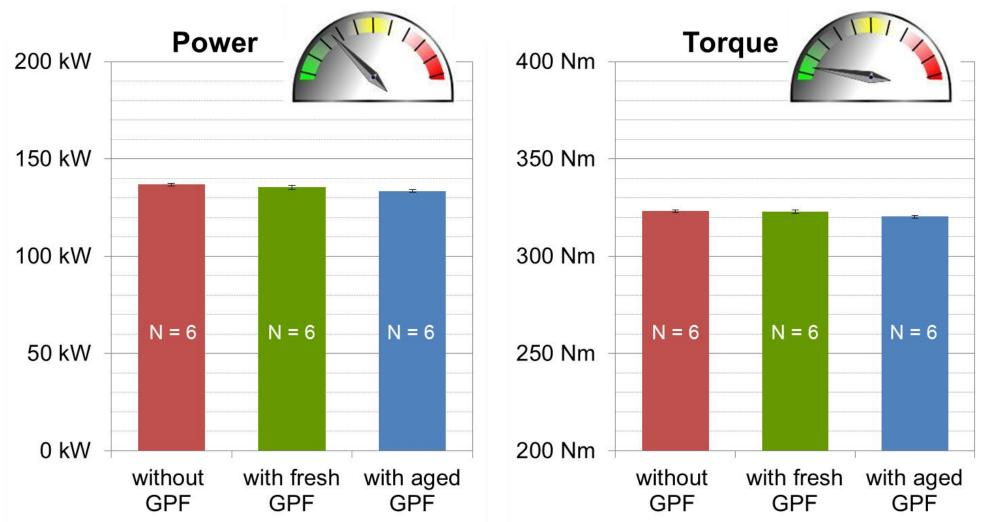
Less than 3% power loss and torque loss with aged GPF is observed during wide open throttle acceleration.
