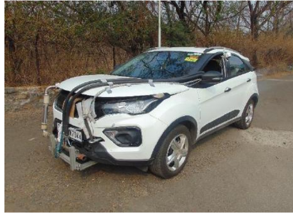
PEMS at Vehicle Inlet
