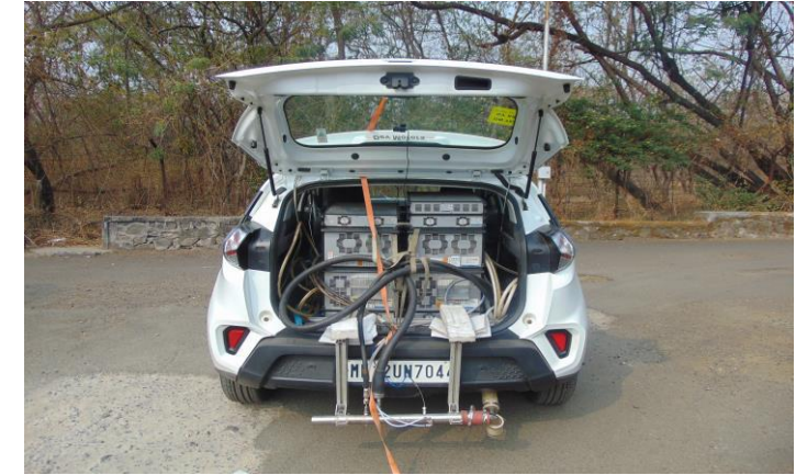
PEMS at Vehicle Tail pipe
