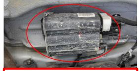
activated carbon canister (ORVR on large-scale factory-produced U.S. Fiat 500)
