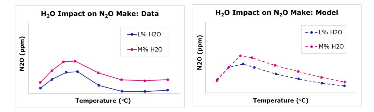
• Model applicability extended to  $H_2$ -ICE conditions; update completed to better predict the impact of  $H_2O$  content in exhaust gas mix on  $N_2O$  selectivity
