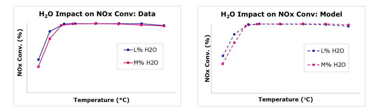
• Model applicability extended to  $H_2$ -ICE conditions; update completed to better predict the impact of  $H_2O$  content in exhaust gas mix on NOx conversion
