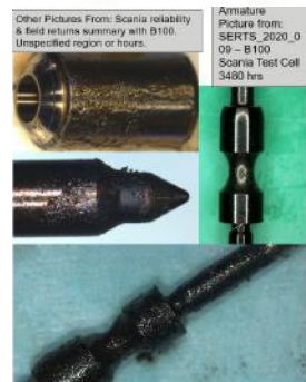
Injector deposits primarily from poor condition fuel
