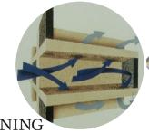
Wall flow mechanism traps exhaust particulates
