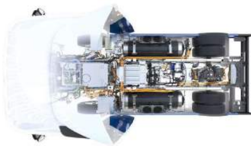
Fig. 8. The final powertrain integration of AVL's fuel cell demo truck. (© AVL)
