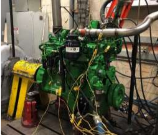
John Deere 6068 (6.8L) Tier 4f Engine
